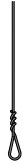
Pre-stressed wire \varnothing \geq 2.0 mm; fixing ends are bound at least 3 times
